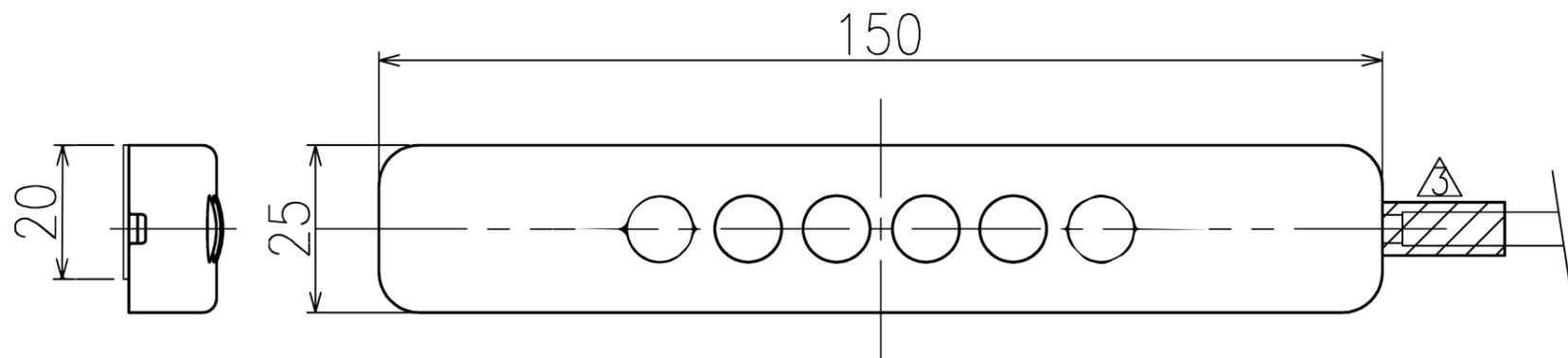
SWP-TYPE CONNECTOR SEAL RUBBER 1P ASSY (7157-7811-80)
